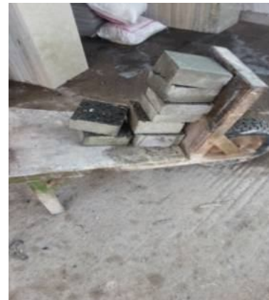
Fig 2. Concrete samples cut in stonework factory
